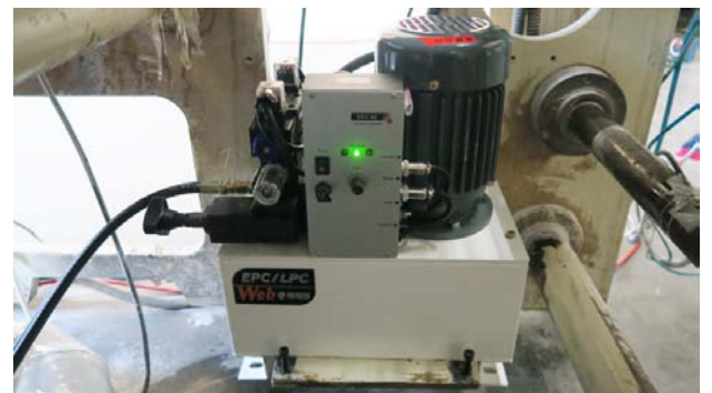
Controller Series 66 is installed on TOUGU DENKI Hydraulic Actuator directly
